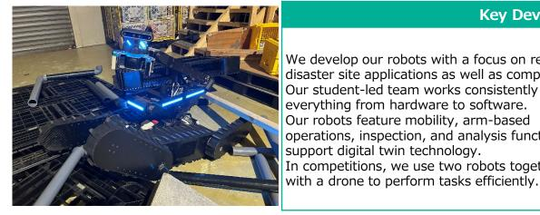
We develop our robots with a focus on real disaster site applications as well as competitions. Our student-led team works consistently on everything from hardware to software. Our robots feature mobility, arm-based operations, inspection, and analysis functions to support digital twin technology. In competitions, we use two robots together
