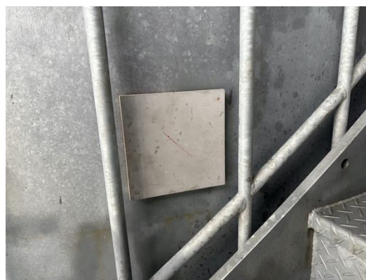
Figure 2: Example of an Installed Board Test Piece - Tank
